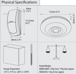
PD 6662 & EN 50131 Grade 3 Environmental Class II. Conforms to European Union (EU) Electro-Magnetic Compatibility (EMC) Directive 89/336/EEC (amended by 92/31/EEC & 93/68/EEC). Approved to BS EN 55022 Class B & BS EN 50130-4: 1996. The CE mark indicates that this product complies with the European requirements for safety, health, environmental & customer protection. Premier Elite is a trademark of Texecom Ltd. © 2012 (LIT-0164)
